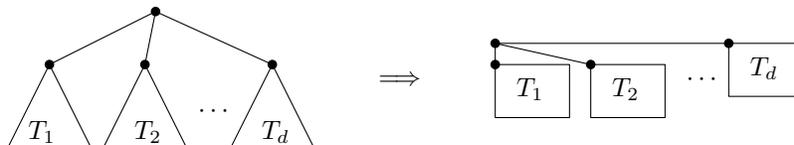
Figure 2: The “standard” algorithm to produce a straight-line upward drawing of any tree of size  $n$ , with width at most  $n$  and height at most  $\lceil \log n \rceil$ : reorder the subtrees so that  $T_d$  is the largest, then recursively draw  $T_1, \dots, T_d$ .
