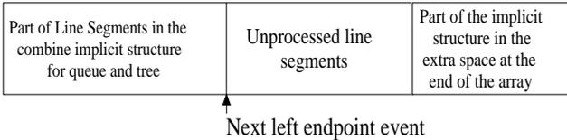
Figure 1: The memory layout of our algorithm.
